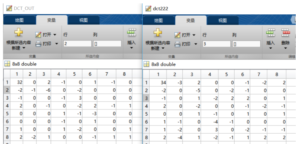
图 3-1 左图为快速算法的输出，右图为 Matlab 自带函数的输出 Fig. 3-1 The left picture is the output of the fast algorithm, the right is the output of Matlab's own function
